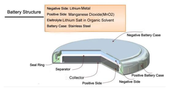
Chemical System: The coin type lithium manganese dioxide battery uses lithium as the negative active material, MnO2 as the positive active material, and an organic electrolyte solution.
