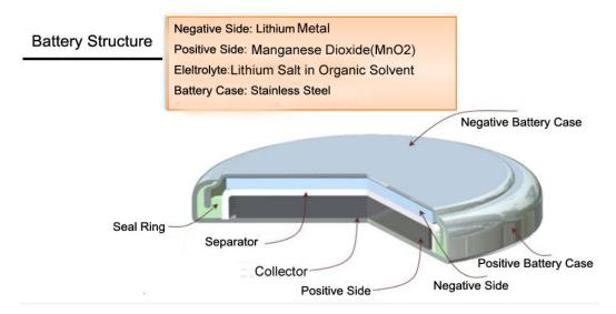
Chemical System: The coin type lithium manganese dioxide battery uses lithium as the negative active material, MnO2 as the positive active material, and an organic electrolyte solution.
