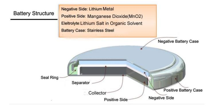
Chemical System: The coin type lithium manganese dioxide battery uses lithium as the negative active material, MnO2 as the positive active material, and an organic electrolyte solution.
